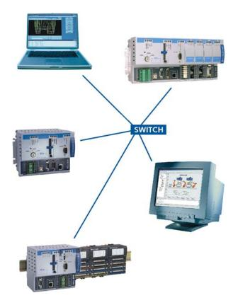
You can connect several controllers directly via global PLC variables, or via a PC network. OPC servers run the communication with standard visualizing and operating programs.
