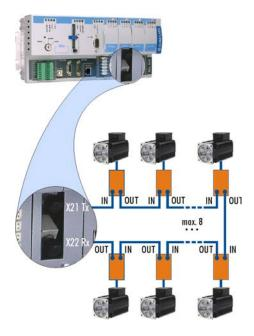
The Sercos XP-SRC drive module XP-SRC(x) provides a Sercos ring on which up to 2, 4, 6 or 8 independent Sercos drives can be operated via optical fiber.
