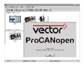
The ProCANopen program allows convenient configuring of the CANopen network on a PC under Windows. ProCANopen is suitable for systems with a central controller (master-slave architecture) as well as for
