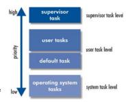
to process it. This means that valuable performance is not wasted in unnecessary waiting cycles. Furthermore, the tasks are assigned different priorities that ensures they are processed in order of importance.
