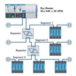
Using the XF-DPM field bus module makes the XCx into a class-1-master in a Profibus-DP network. Parallel operation with the CANopen field bus is possible.
