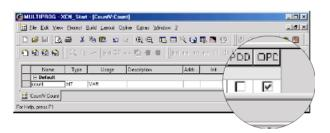
In the variable dialogs on Multiprog the controller data and variables where the OPC server requires read/write access are simply designated OPC ( $\rightarrow$  page 14).
