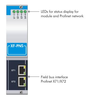
Using the interface module XF-PNS XCx controllers can be integrated in networks with higher-level Profinet controllers for distributed operation. Real-time data exchange between master and slave as well as slave and master is done using configurable arrays.
