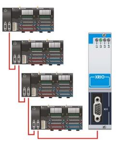
The XRIO interface module provides an additional connection for four interface modules (RIO EC X2 for RIO modules, XBXC for XCx micro modules) each with eight digital or analog I/O modules, in addition to the standard integrated XRIO connection. A high-speed protocol without field bus delay controls the modules via the serial interface.
